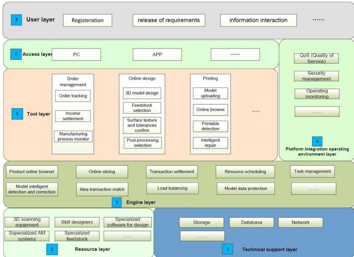
[그림 1] Typical system framework of AMSP
